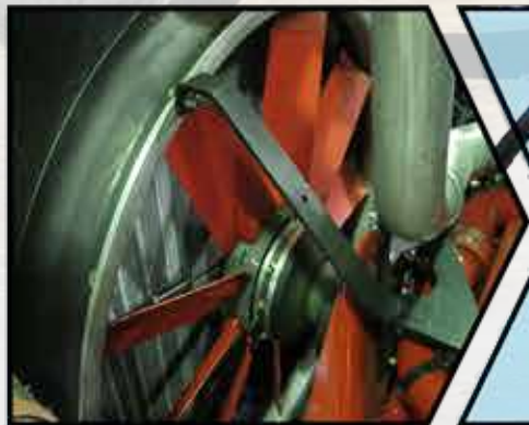
Reversible Fan Fan automatically cycles between pull and push modes reducing dirt and debris buildup in radiator.
