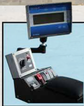
Control Console All mixer controls at your fingertips. Ergonomic design includes central location for all fuses and relays.
