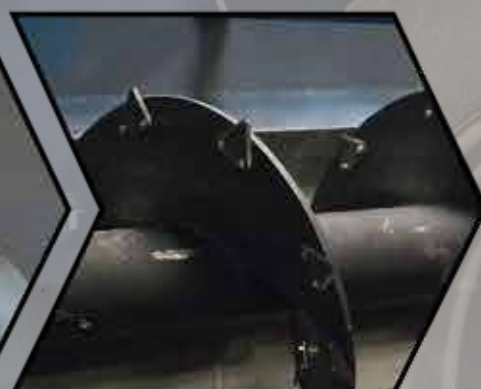
Top Auger Knives Improve break up and incorporation of bulky ration ingredients.
