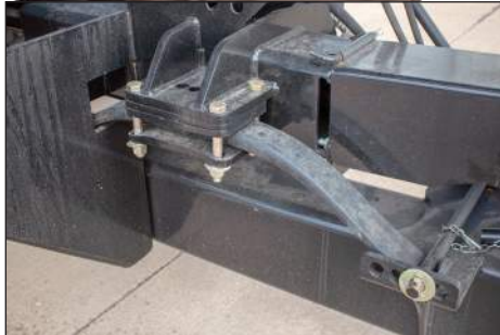
Spring Suspension Tongue - smother ride loaded/unloaded - evens weight transfer at higher speeds - adjustable for tonque height
