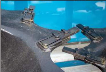
Beater knives are reversible and reinforced to handle tough materials.
