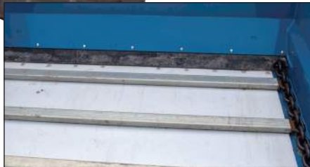
Poly floor and floating galvanized slats provide corrosion resistance. Seals front and back, keep sloppy materials in the spreader
