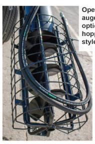
Open intake auger provides options for hopper or pit style unloading
