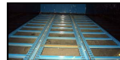
Poly Floor & Sides with Stainless Steel Side & Floor Retainers
